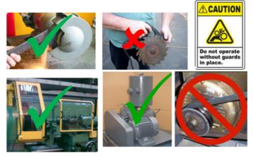
Never tamper with or removed guards from any equipment or tool.
