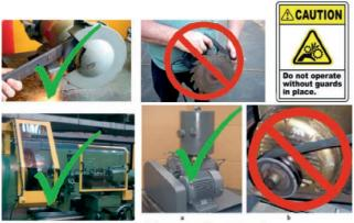
Never tamper with or remove guards from any equipment or tool.
